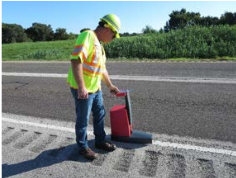
Figure 3. Photo. Measuring retroreflectivity with a handheld instrument.
