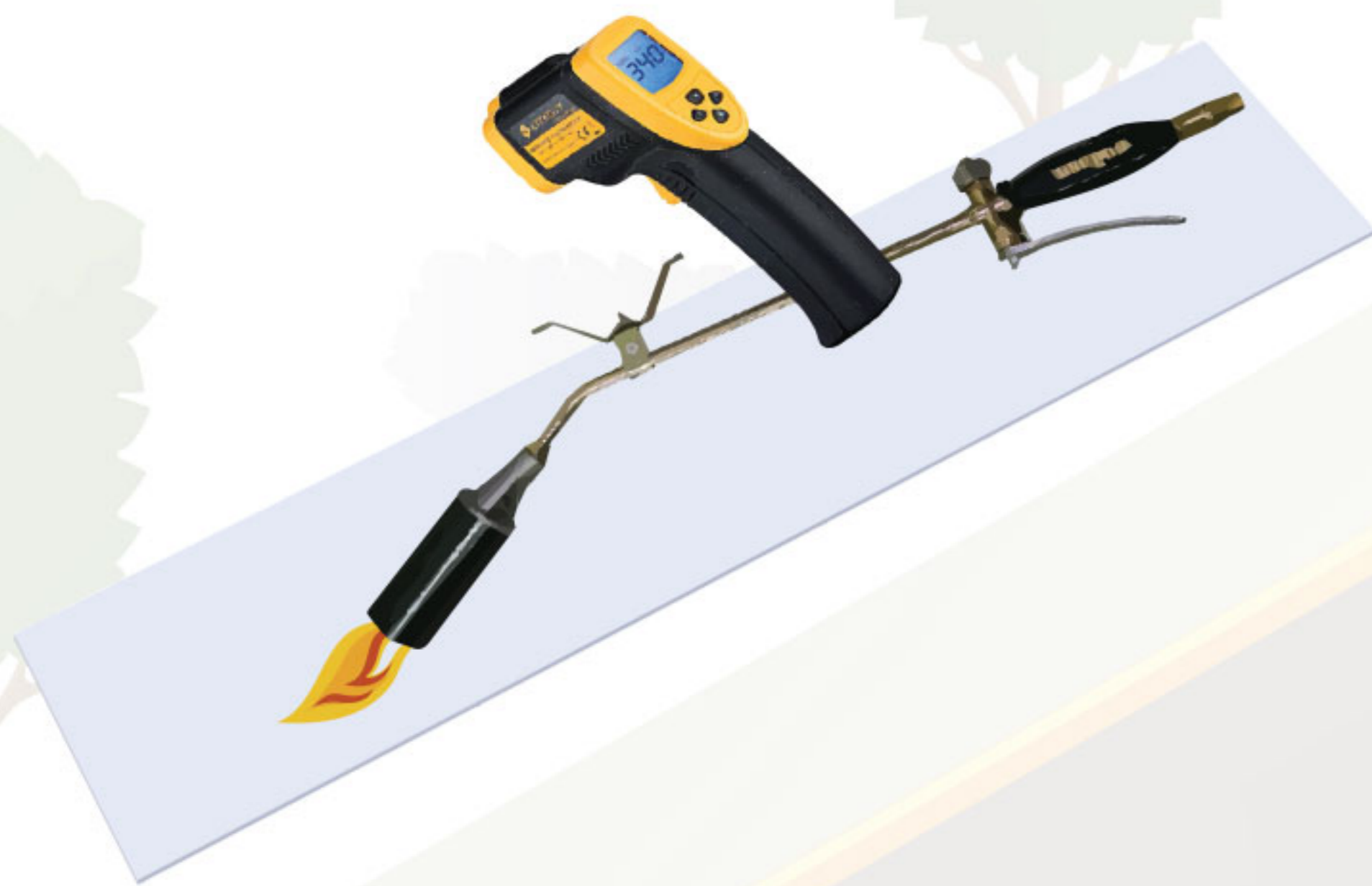
Melt Adhesive Panel to 340°F
